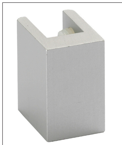
Panel end connector silver coloured, anodized with plastic clamping screws
