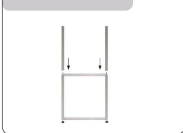
4. Mount the upper aluminium cross profile incl. pointed screws.
