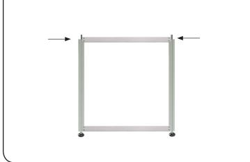
3. Push the top profiles onto the bolts. Ensure that the holes face upward.
