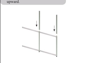
4. Then mount the cross profiles including the pointed screws.
