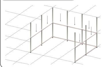
6. Then mount the cross profiles including the pointed screws.
