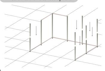
6. Then mount the cross profiles including the pointed screws.
